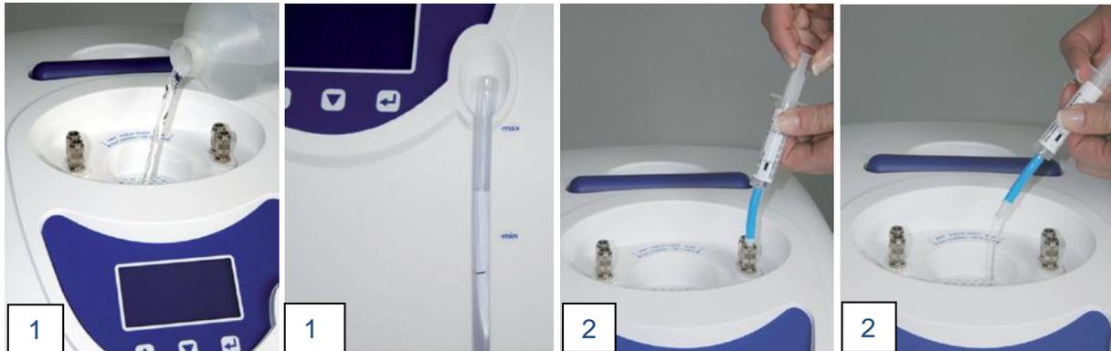
2. Bleed the air from the pump system. To bleed click the deairing set into one of the plug in coupling on the top of the device. It should click into place. Pull the syringe until water is sucked into the deairing set. Remove the deairing set and empty the syringe back into the water tank.
