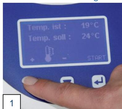
2. Start/stop operation, fill/empty cuffs. To start operation and fill the cuffs press the enter button below the start indication. To stop operation press the enter button below the stop indication.
