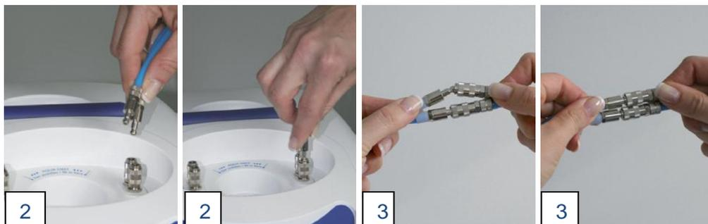
3. Connect cuff(s) to the hose(s). Insert the plug-in nipples of the cuff into the connection couplings of the hose until arresting with an audible click. It doesn't matter which plug is plugged into which coupling.
